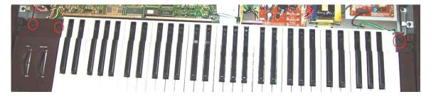
Carefully lift the keybed slightly up and out (toward yourself) an inch or so. You don't need to move it much. You will probably need to free up one or more cables to accomplish it. Or if you prefer, disconnect the cables and completely remove the keybed.
