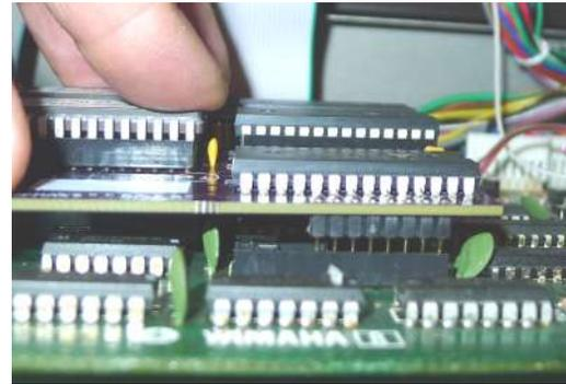
Once you are happy that all the pins are aligning with the desired locations, firmly and evenly press the DX7mega128 board in place. Make a visual check to see that the board is flush with the sockets.
