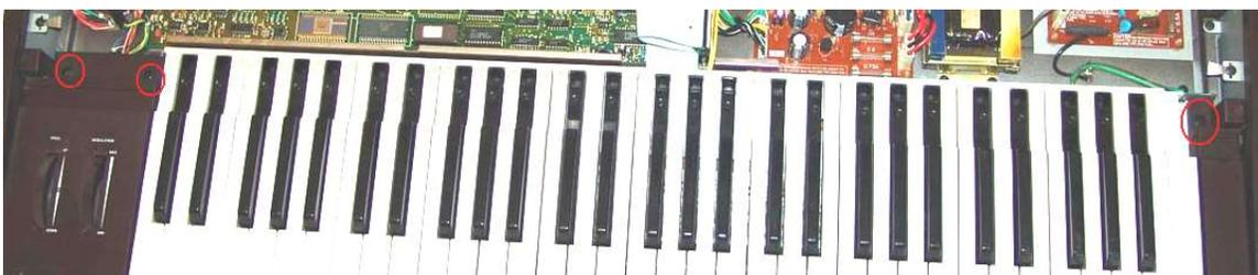
**Carefully lift the keybed slightly up and out (toward yourself) an inch or so..** You don't need to move it much. You will probably need to free up one or more cables to accomplish it. Or if you prefer, disconnect the cables and completely remove the keybed.
