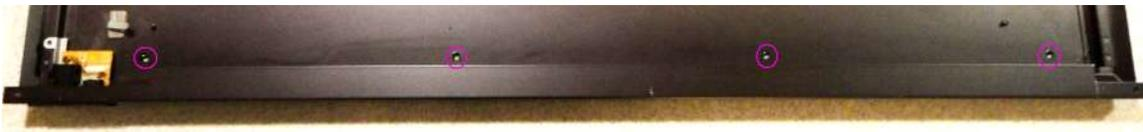
**Loosen the 3 internal screws at the extreme right and left ends that hold the keyboard in place.** It is not necessary to extract them from the holes they reside in.
