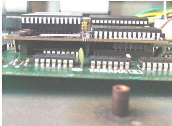
Using a screwdriver, carefully tighten the original main board screw through the DX7mega128 board into the nylon standoff. **Again do not force it or over tighten as this can not only strip the standoff, but it can cause the DX7mega128 board to change position. It should be tight enough so that it cannot work loose.** Double check the pins.
