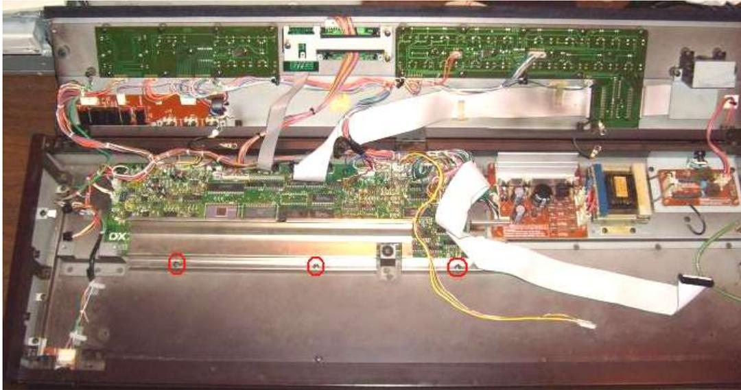
You now have excellent access to the DX7 main board. If you do remove the keybed you may find it easier to remove the small yellow cable and large flat grayish cable at the main-board-end rather than from the keybed. You will also need to unclip two small cables on the left end (mod wheel and pitch bend). There may also be wire tires and/or cable fasteners to deal with.
