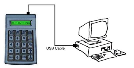
If you are hooking the MIDI Patch Changer keypad to a **PC that has USB**, then you can use the supplied RJ-to-USB cable:
