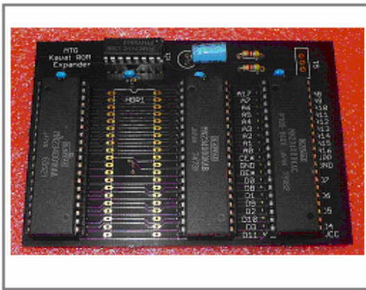
R100 3x ROM Switcher Board
